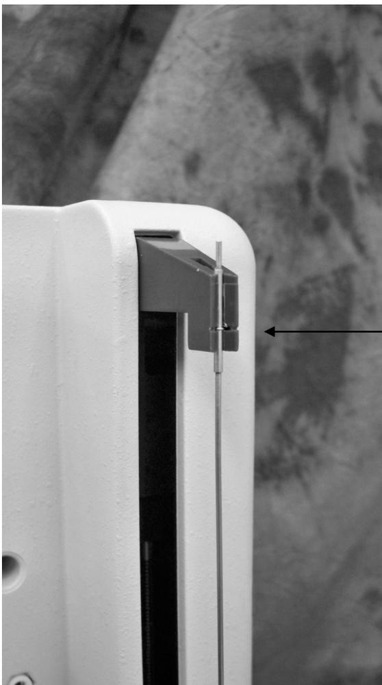
Align collar on probe with notches on probe arm.
